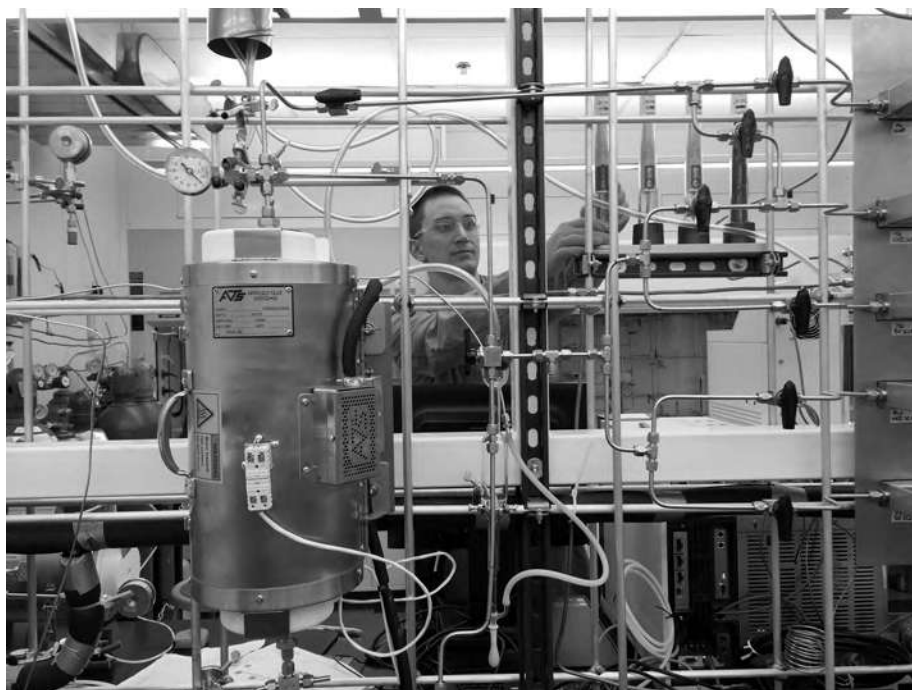
Chemical and Biomolecular Engineering assistant professor Dante A. Simonetti sets up a packed bed reactor.
