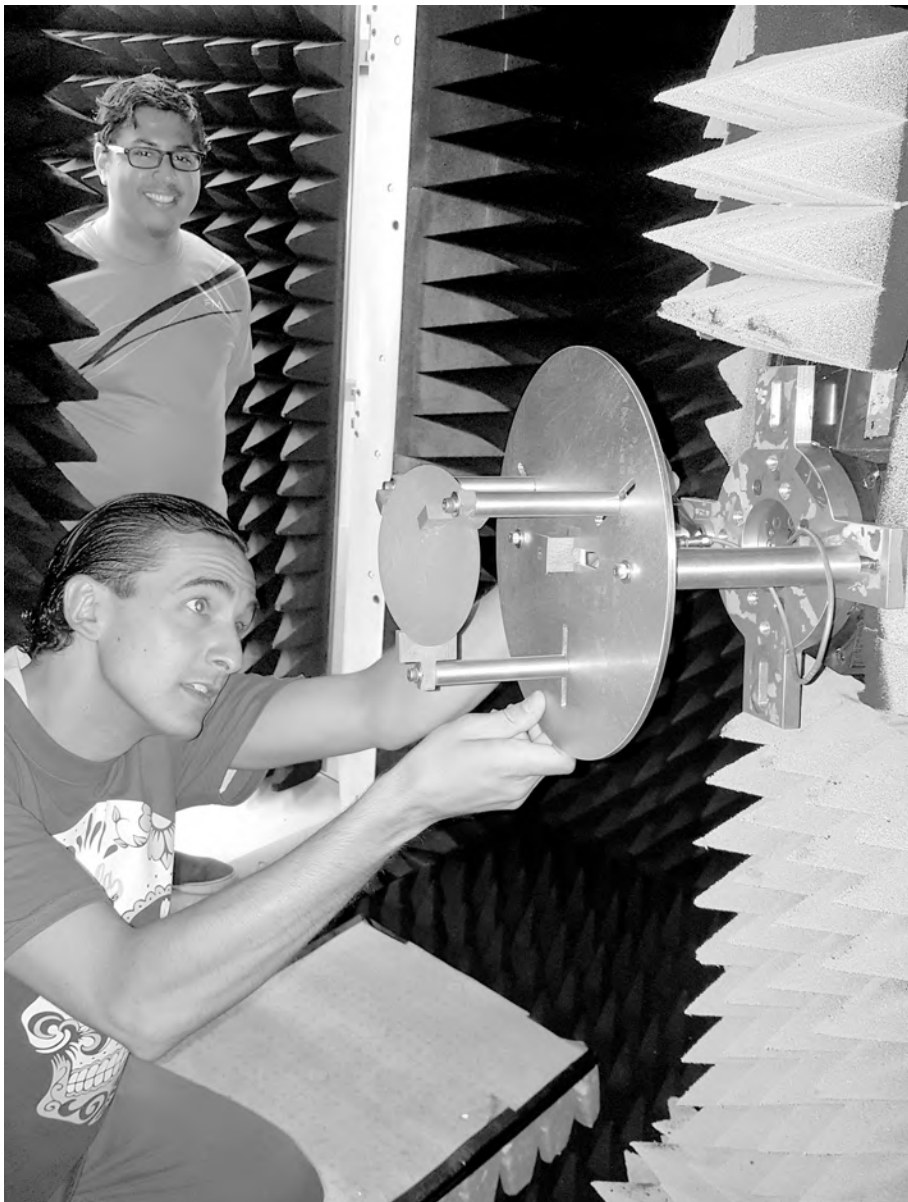
Doctoral student Jordan Budhu and masters student Vignesh Manohar, under the direction of professor Vahya Rahmat-Samii, set up a spherical near-field antenna measurement system to measure the radiation pattern of a lens antenna for potential future space applications.
