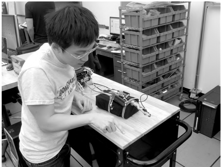
Cheng-Ju (Jimmy) Wu describes the BairClaw robot hand testbed in associate professor Veronica J. Santos' Biomechatronics Laboratory.
