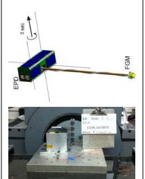
Top: UCLA CubeSat "Elfin" (concept). Bottom: Elfin instrument suite during vibe-tests, to be launched as a piggyback aboard Russian Lomonosov satellite (delivered: July 6).
