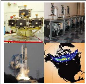
THEMIS consists of 5 spacecraft (top left) in orbit since 2007 (launch: bottom left) and a geophysical network of >20 ground magnetometers / auroral imagers (top right) in operation. UCLA is this NASA mission's PI institution.
