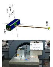
Top: UCLA CubeSat "Elfin" (concept). Bottom: Elfin instrument suite during vibe-tests, to be launched as a piggyback aboard Russian Lomonosov satellite (delivered: July 6).
