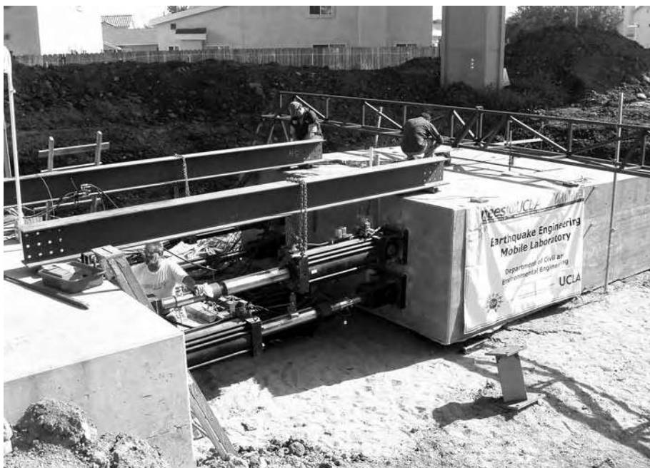
Full-scale test of a bridge foundation system subjected to simulated earthquake loading at the UCLA/Caltrans field test site near Los Angeles International Airport (LAX).
