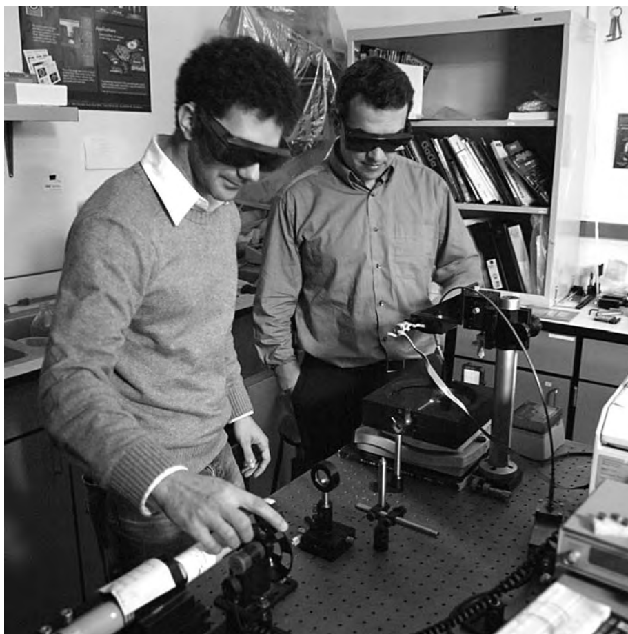
Professor Laurent Pilon and Ph.D. student Halil Berberoglu measure the optical properties of carbon dioxide-consuming and hydrogen-producing algae.
