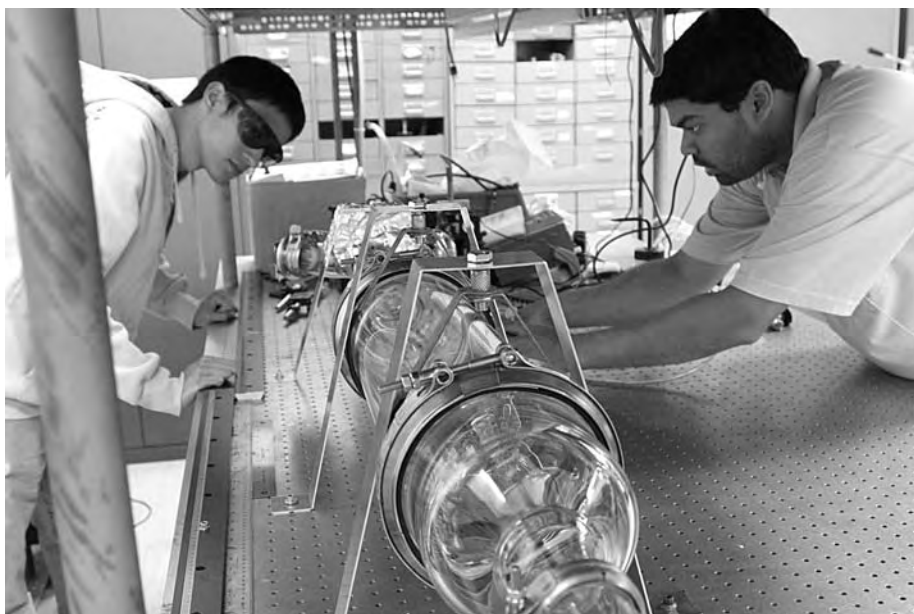
Students assemble an apparatus to measure laser scattering in fog.
