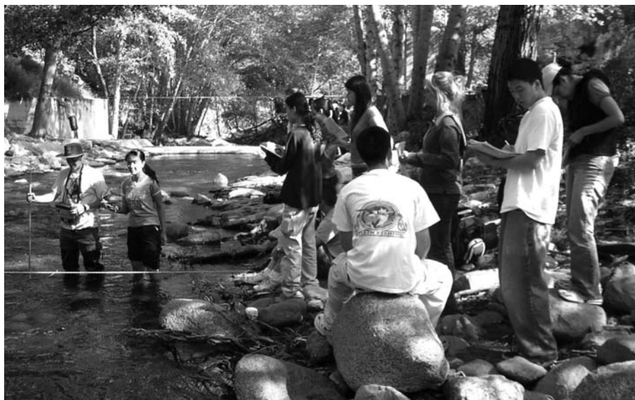
Civil and Environmental Engineering students learn streamgauging in the Arroyo Seco channel as part of the Hydrologic Analysis and Design course.
