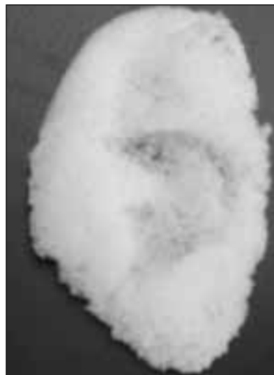
Complex-shape microporous scaffold for tissue engineering
