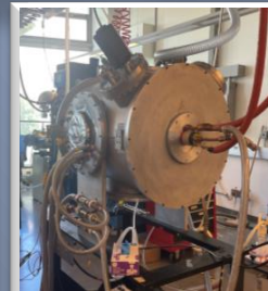
Fig. 4 Partially assembled vacuum chamber with our High Energy Flux Test Facility (HEFTY) attached.
