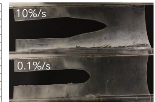
Figure 10. Different crack tip shapes observed at fast and slow loading rates
