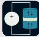
Fig. 1 – VC-MTJ Module Uses the fixed layer on the bottom as a reference to detect whether the device is parallel, "0" or antiparallel, "1"
