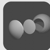
Fig 5. Deconstructed view of the mesh that makes up our eye model (cornea, iris, sclera from left to right)
