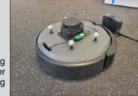
Figure 2: Robot moving with LiDAR scanner measuring surrounding environment
